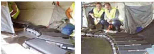
Elastīgais transportieris „Rampsnake” (avots: FlightCare Belgium)
