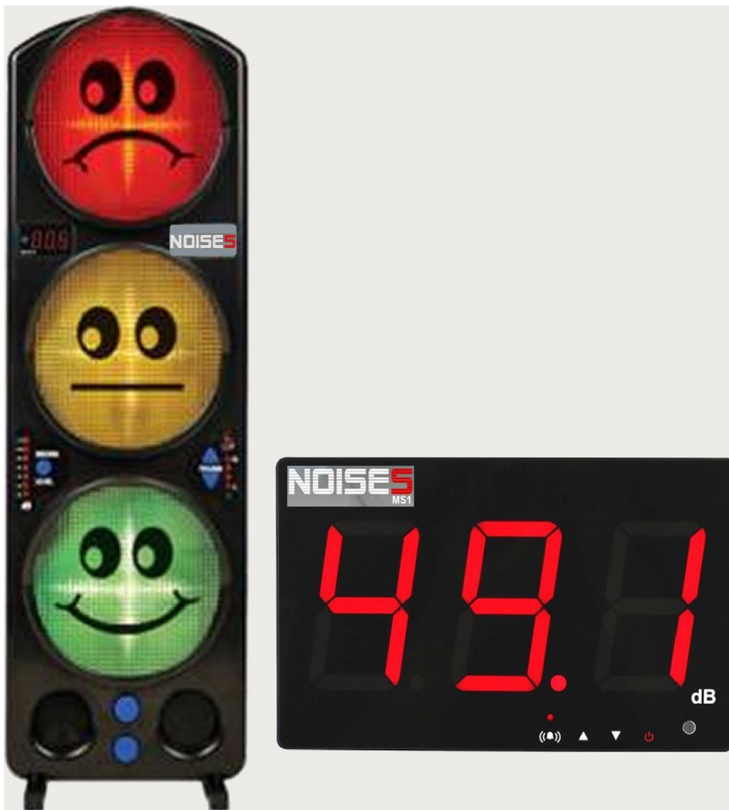
Figure 1. Noise meter which emits a visual and auditory alarm and a digital noise meter
