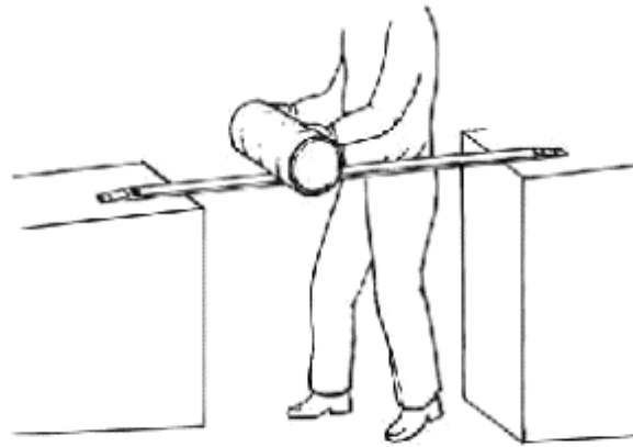
Slides can be configured at low cost in spots where standard conveyors do not fit.
