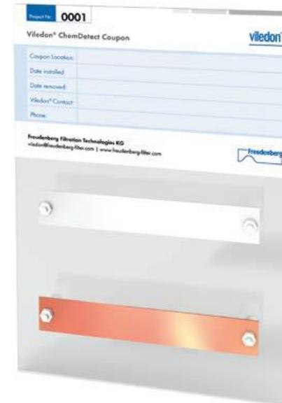
The Viledon® ChemWatch Online Monitoring System determines the corrosion class of gaseous media in accordance with standard ANSI / ISA-71.04-2013. The system calculates the corrosion rate (copper and silver), temperature, relative air humidity and the positive pressure in the room to allow a targeted analysis.
